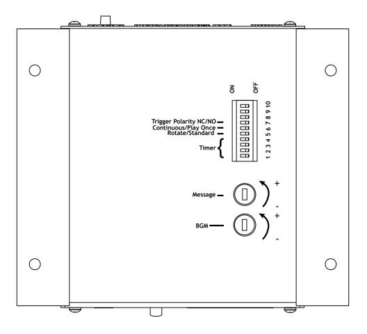
BGM - This pot is used to control the final output level of the background music that is fed through the units BGM INPUT on the I/O CONNECTOR on the rear of the unit. Volume up is counter-clockwise, volume down is clockwise.
